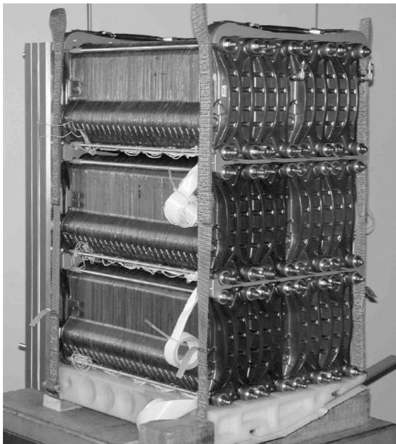
Figure 3: Array of six stacks of 125 cells with manifolding plate (below and left side). Total weight 185 kg.
